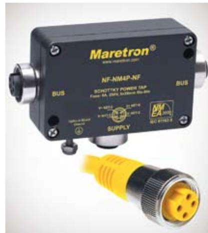
A Powertap is connected to a network backbone just like any Tee but rather than connecting a device, its purpose is to provide "bus" power. Typically a Powertap is placed as central as possible between total devices on backbone. Maretron Powertap uniquely provides two power inputs permitting doubled power provision for devices.
