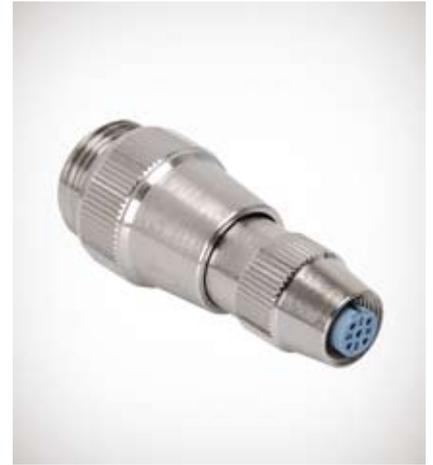
The reducer is used to change from a Mini cable to Micro or Mid cable. For example, one end of the network might be terminated at the top of the mast but it may not be desirable to run a Mini trunk cable up the mast. In this case, you can switch over to Micro or Mid cable at the base of the mast using the reducer and continue up the mast with Micro or Mid cable.
